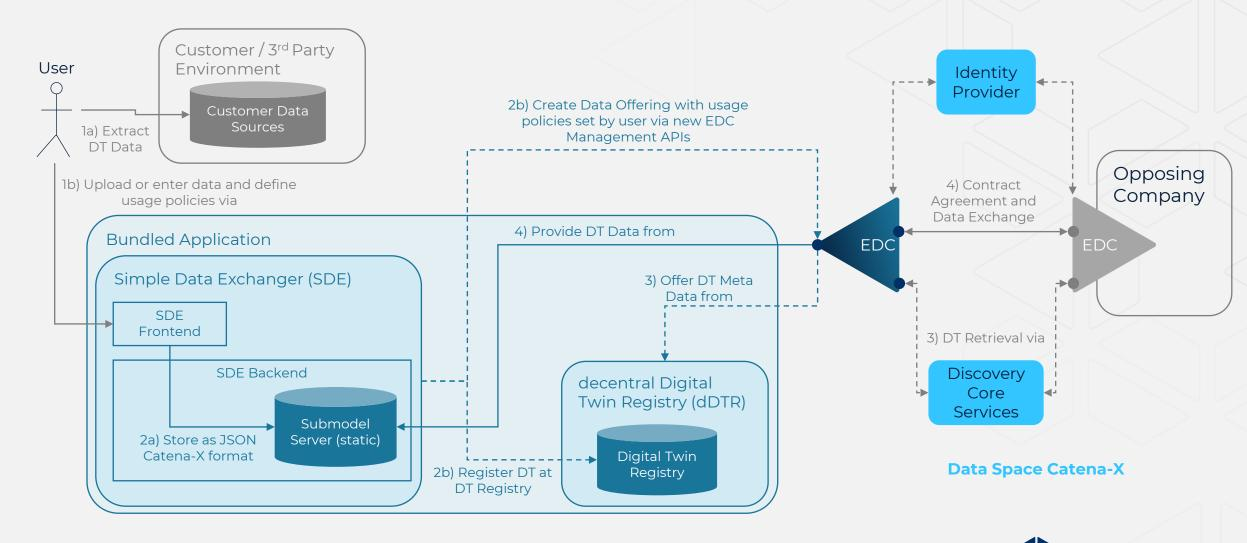
DT = Digital Twin, dDTR = decentral DT Registry, EDC = Eclipse Data Space Components Connector, IP = Identity Provider, SDE = Simple Data Exchanger
